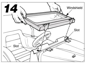
• Fit the tabs on the back of the windshield into the slots in the dash.
